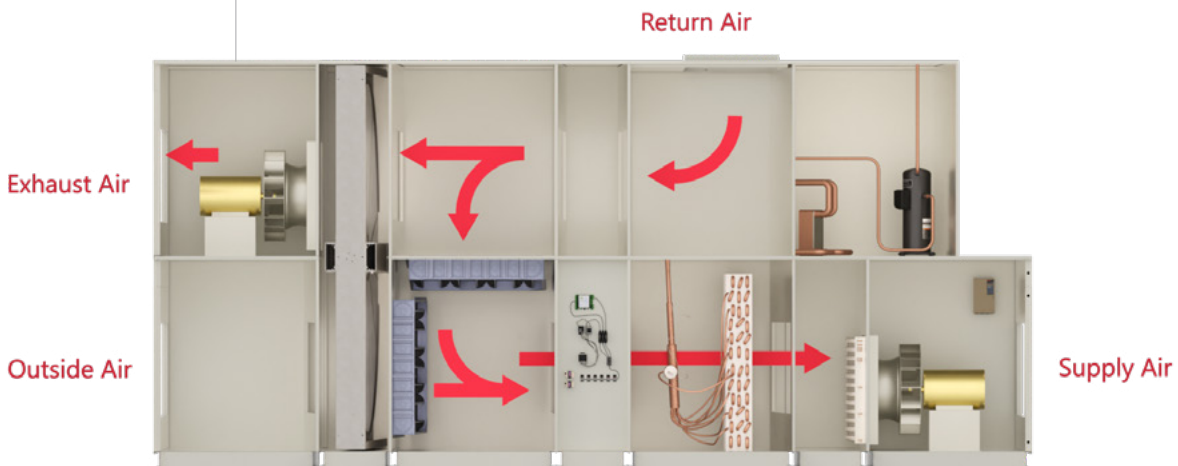
Energy Recovery Unit with Water-Source Heat Pump, Economizer and Electric Heat Strips
