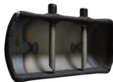
Figure 96 - Horizontal Receiver Internals
