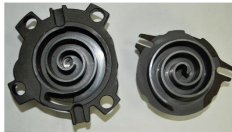
Top fixed scroll Bottom orbiting scroll
