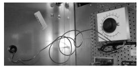
Figure 15 - Adjustable compressor lockout
