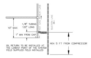
Figure 26 - Hot Gas Purge Circuit
