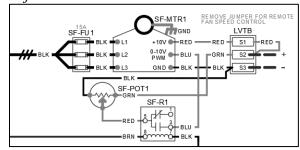
Figure 20 - Typical wiring diagram with EC motor
