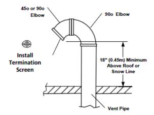
Figure 39 - Open Combustion Venting
