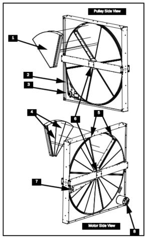
Figure 29 - Polymer Energy Recovery Wheel
