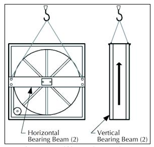
Figure 28 - Lifting Hole Locations
