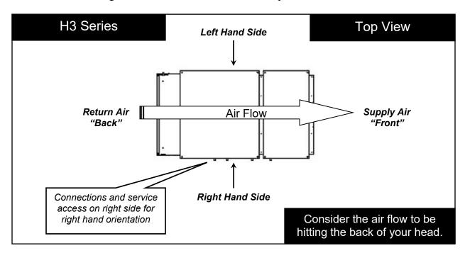
Figure 7 - H3 Series Unit Orientation
