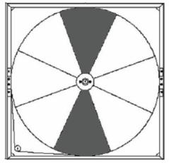
Figure 30 - Wheel Segment Removal Pattern
