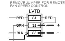
Figure 21 - Shows the jumper that is to be removed (jumped between S1 and S2).
