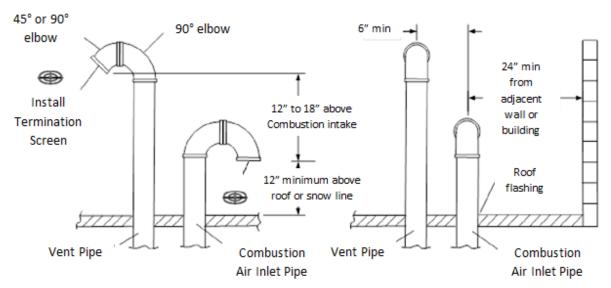
Figure 41 - Separated Combustion Venting
