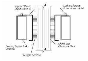
Cross Section of Air Seal Structure
