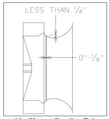
Figure 19 - Plenum Fan Gap Tolerances
