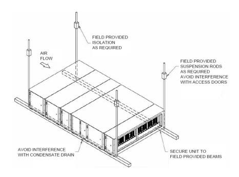
Figure 6 - H3 Series Parallel Beam Suspension Installation
