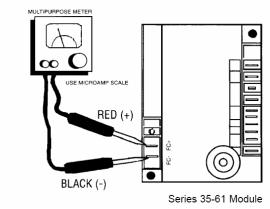
Figure 46 - Flame Sensor Current Check
