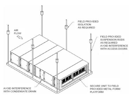
Figure 5 - H3 Series Platform Suspension Installation
