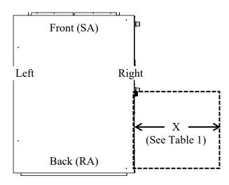
Figure 3 -Minimum Clearance Required for Access to Unit (H3 Series plan view)
