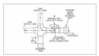
Figure 42 - Sediment Trap for Gas Heat
