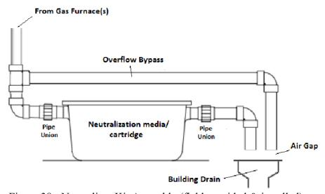
Figure 38 - Neutralizer Kit Assembly (field provided & installed)
