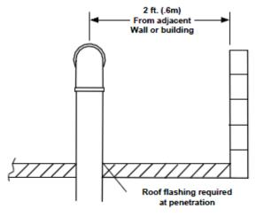
Figure 40 - Open Combustion Venting
