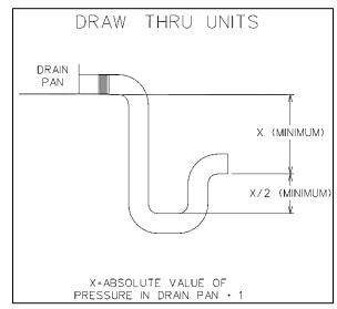
Figure 18 - Drain Trap
