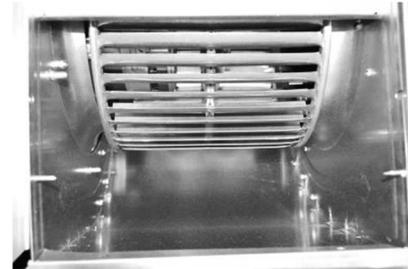
Figure 11 - WSHP Series Supply Fan
