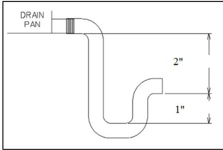
Figure 6 - Drain Trap
