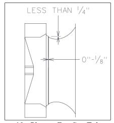
Figure 10 - Plenum Fan Gap Tolerances
