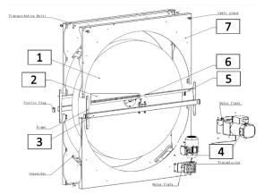
Figure 14 - Aluminum Energy Recovery Wheel
