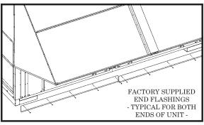
Figure 6 - Factory Supplied End Flashings
