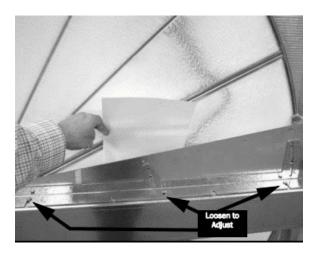
If it is necessary to adjust a purge seal to the face of the wheel, loosen the two or three screws along the bearing beam and adjust to the proper distance from the media surface. Tighten the screws and retest the seal.
