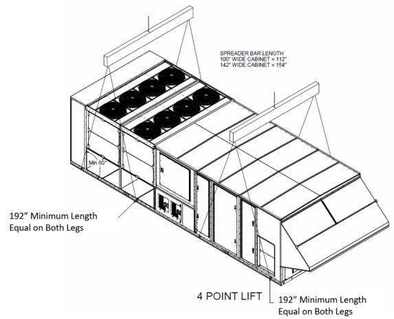
Figure 3 - Lifting Details of a 75-140 ton Unit
