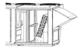
Figure 11 - Evaporator Coil Access
