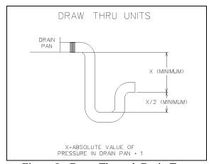
Figure 9 - Draw-Through Drain Trap
