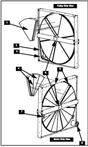
Figure 16 - Polymer Energy Recovery Wheel
