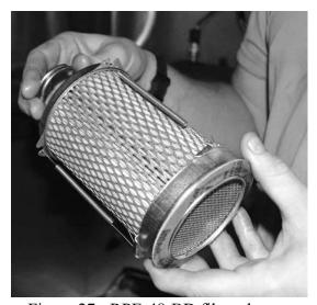
Figure 27 - RPE-48-BD filter element
