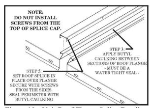
Figure 10 - Unit Roof Flange Splice Detail
