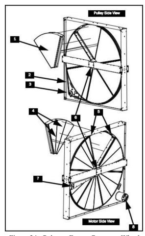
Figure 34 - Polymer Energy Recovery Wheel
