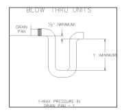
Figure 18 - Blow-Through Drain Trap
