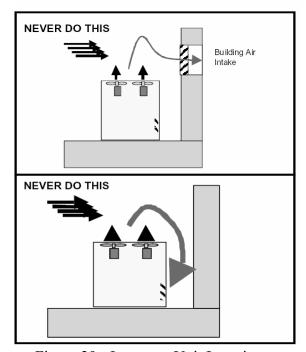
Figure 29 - Improper Unit Locations
