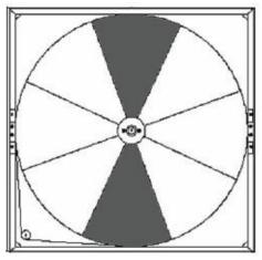
Figure 35 - Polymer Wheel Segment Removal Pattern
