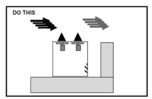
Figure 28 - Proper Unit Location
