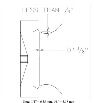
Figure 23 - Plenum Fan Gap Tolerances
