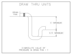
Figure 17 - Draw-Through Drain Trap
