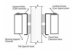
Cross Section of Air Seal Structure
