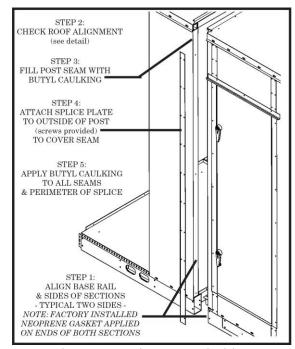
Figure 9 - Unit Base and Sides
