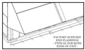
Figure 13 - Factory Supplied End Flashings
