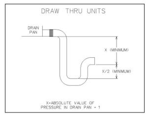
Figure 11 - Drain Trap
