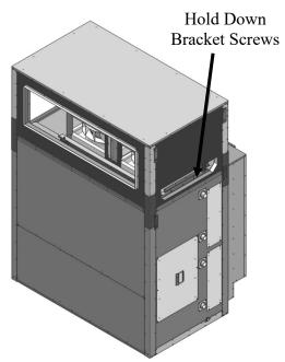
Figure 19 - Back View with Supply Fan Access
