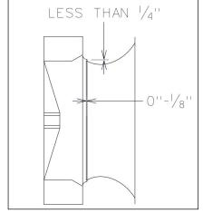
Figure 17- Plenum Fan Gap Tolerances
