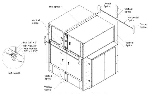
Figure 9 - Dual Unit Assembly Details
