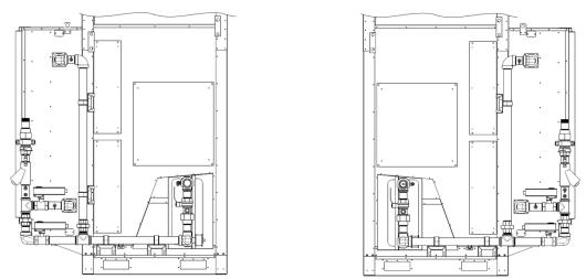
Figure 14 - Air Conditioner Waterside Economizer Back View
