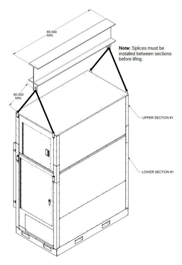
Figure 2 - One Piece Single Unit Lifting Details
