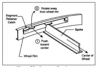
Figure 22 - Segment Retainer
