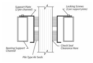
Figure 16 - Cross Section of Air Seal Structure
