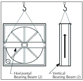
Figure 17 - Lifting Hole Locations
