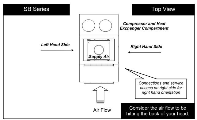
Figure 3 - SB Series Unit Orientation
