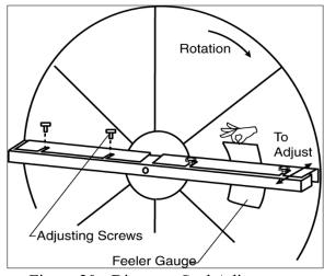
Figure 20 - Diameter Seal Adjustment
