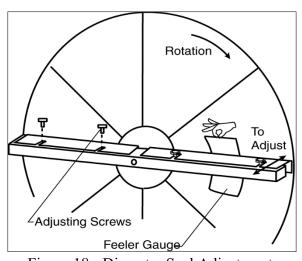
Figure 18 - Diameter Seal Adjustment
