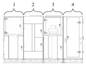
Figure 4 - SB Schematic with (1) Exhaust Fan, (2) Energy Recovery, (3) Air Handler, and (4) Compressor Section
