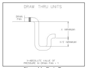
Figure 14 - Drain Trap
