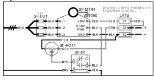
Figure 25 - Typical wiring diagram with EC motor
