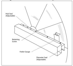
Figure 21 - Hub Seal Adjustment
