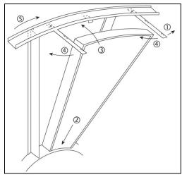
Figure 23 - Segment Installation
