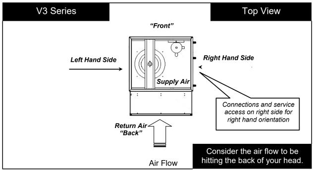
Figure 6 - V3 Series Unit Orientation
