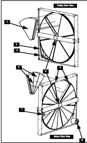
Figure 27 - Polymer Energy Recovery Wheel
