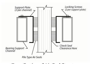
Cross Section of Air Seal Structure
