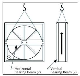
Figure 26 – Lifting Hole Locations
