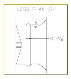
Figure 18 - Plenum Fan Gap Tolerances
