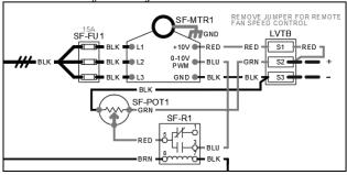
Figure 19 - Typical wiring diagram with EC motor
