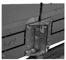
Figure 13 - Forklift Base Assembly
