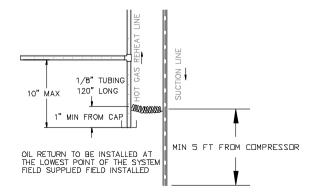
Figure 25 - Hot Gas Purge Circuit
