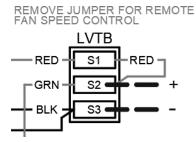
Figure 20 - Shows the jumper that is to be removed (jumped between S1 and S2).
