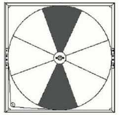
Figure 28 - Wheel Segment Removal Pattern
