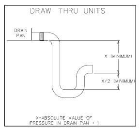
Figure 17 - Drain Trap
